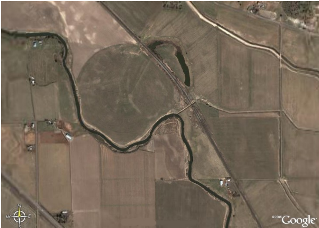
Figure 5. Lost River above Merrill, Oregon with a simplified channel lacking any riparian zone or any connection to wetlands. Old oxbow (above center) isolated by filling. From Google Earth.
