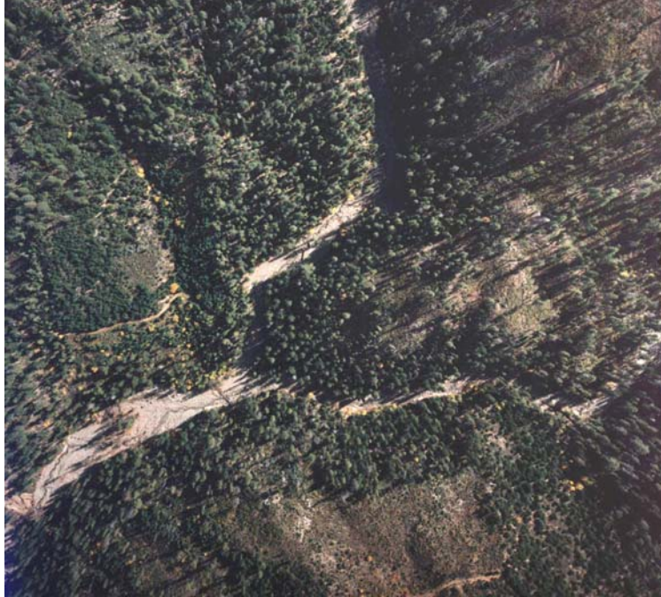
Figure 14. Flow of Walker Creek is barely visible in this March 1997 photo due to massive sediment deposits stemming from debris torrents and crossing failures on January 1, 1997. Channel widening made the stream much more subject to warming. KRIS V 3.0.
