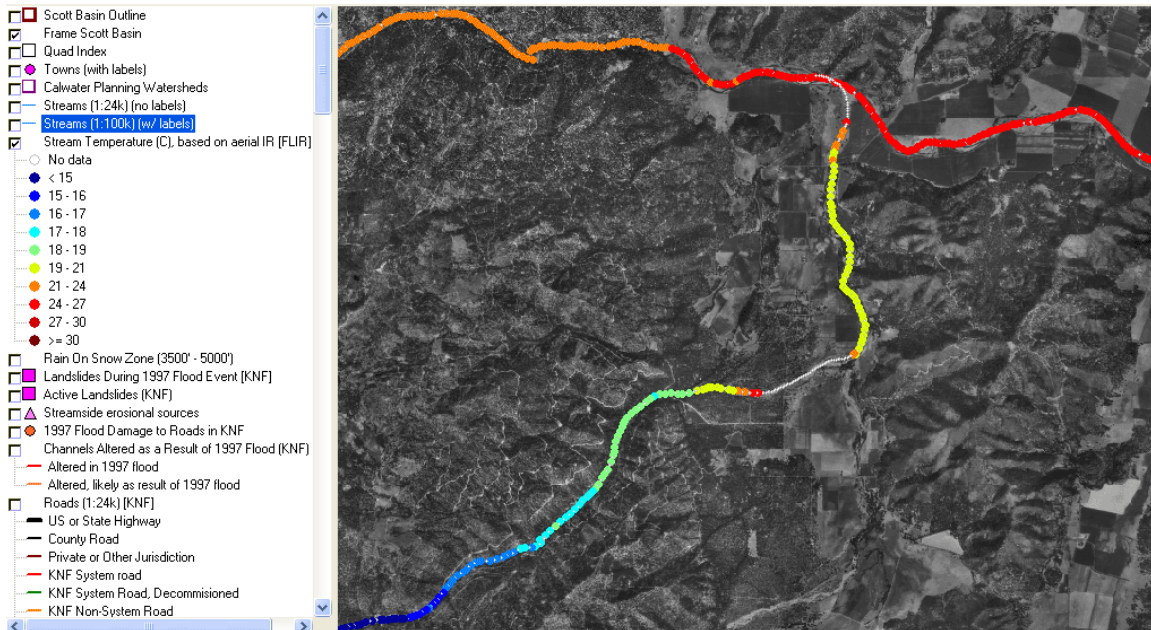
Figure 15. This map shows summary data of Scott River Thermal Infrared Radar (TIR) surveys for Shackleford Creek. Note that water temperature warms in a downstream direction as flow is depleted. Reaches with no temperature coded color (i.e., gray) are dry. Data from Watershed Sciences (2003).
