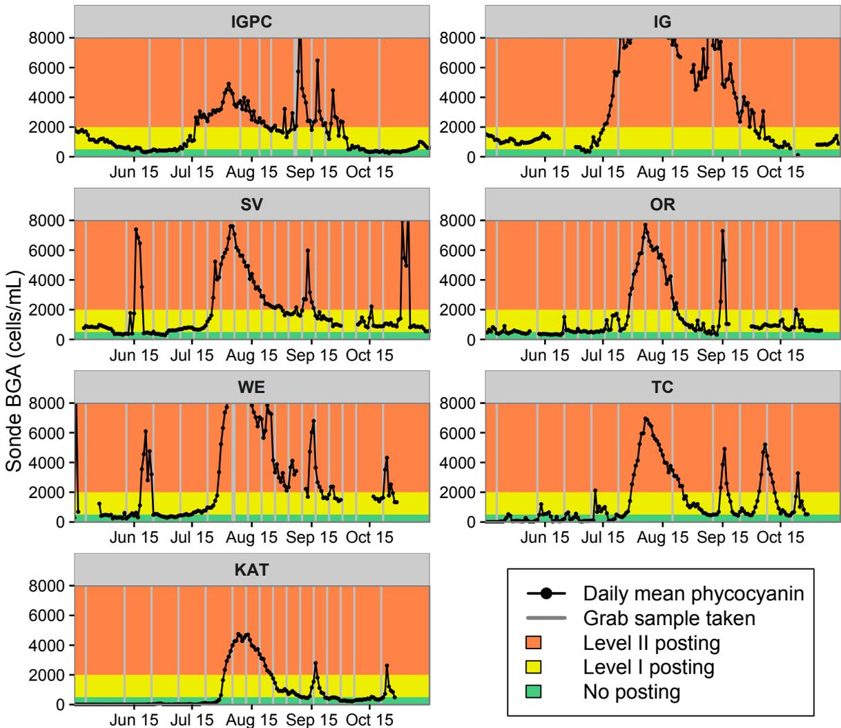
Figure 12. Mean daily sonde BGA at Klamath River sites during 2014 as reported from YSI phycocyanin probes. Background colors indicate possible risk levels as determined from probability of exceedance analyses. Green < 500 cells/mL; Yellow > 500 cells/mL and < 2000 cells/mL; Orange > 2000 cells/mL. Grey vertical lines indicate when grab samples were collected.
