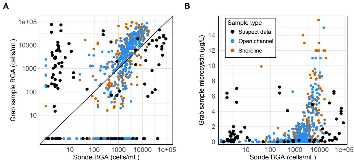
Figure 4. Grab sample BGA (cells/mL, panel A) and grab sample microcystin ( $\mu\text{g/L}$ , panel B) by sonde BGA for all sites and years. Brown points are shoreline grab samples, blue points are open channel grab samples, and black points are grab samples of either type taken on days when sonde data was flagged as suspect.
