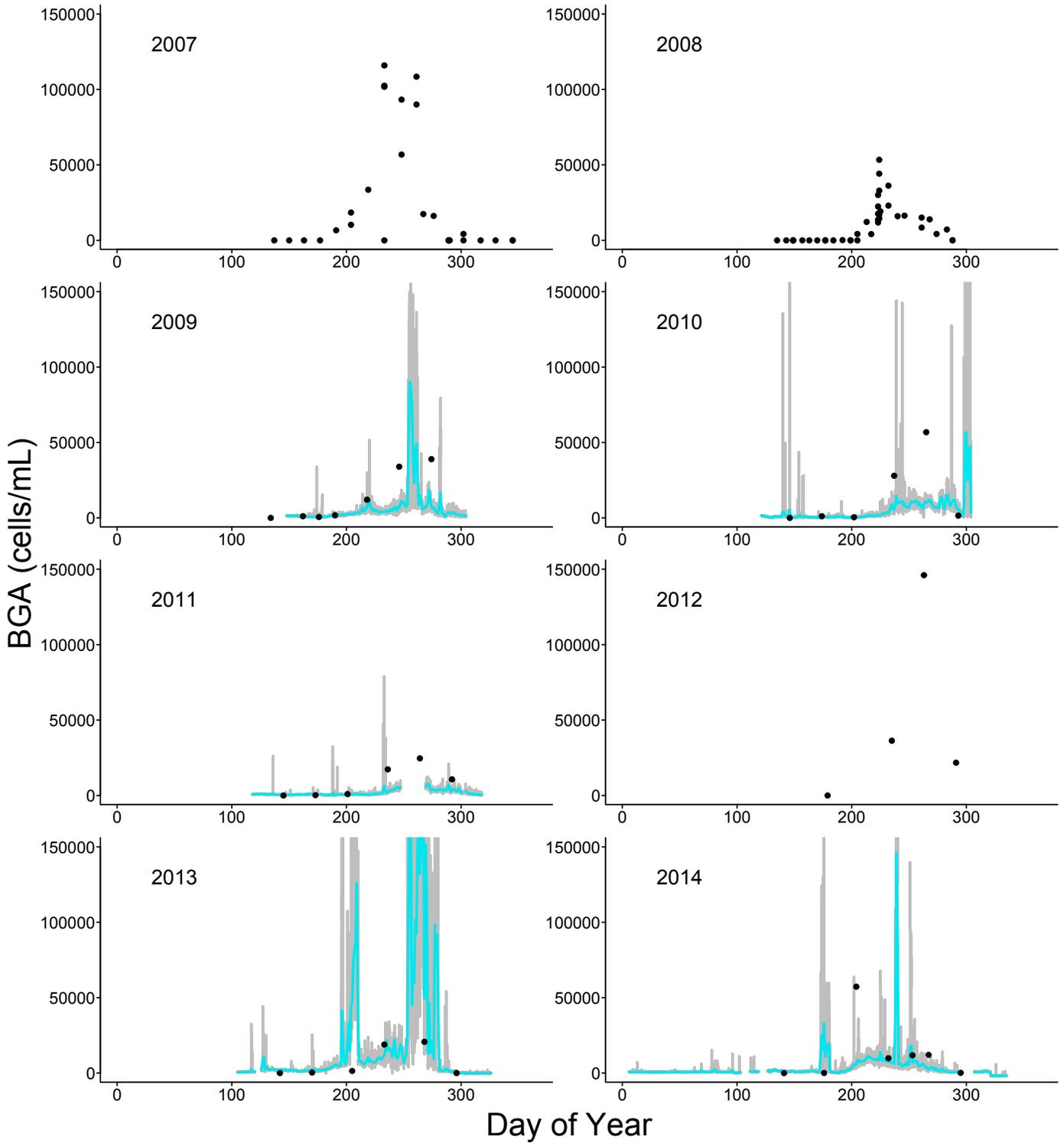
Figure A 2. Raw data (light grey lines) and daily means (blue line) of blue-green algae (bga) cell density estimates from the phycocyanin probe located below Iron Gate dam, operated by the Karuk Tribe. Black points indicate bga cell density from grab samples taken near the sonde location.
