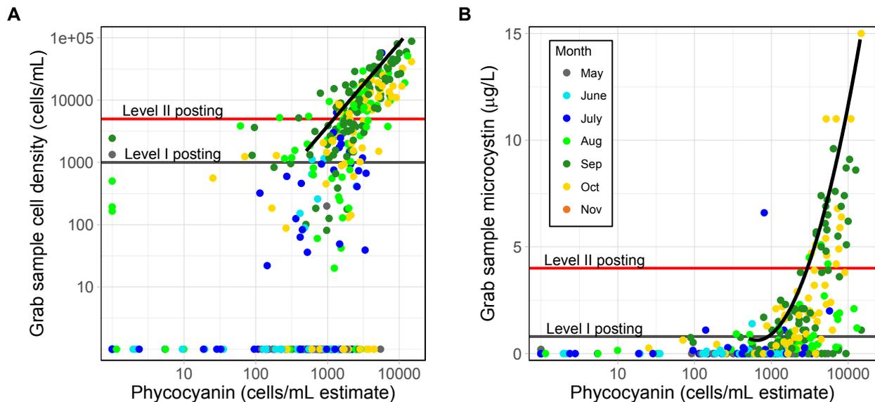
Figure 9. BGA cell density (panel A) and microcystin concentration (panel B) from grab samples by sonde BGA. Colors indicate month during which sample was collected. Black line is the 0.9 quantile regression, and horizontal lines indicate level I and II Tribal health posting threshold.
