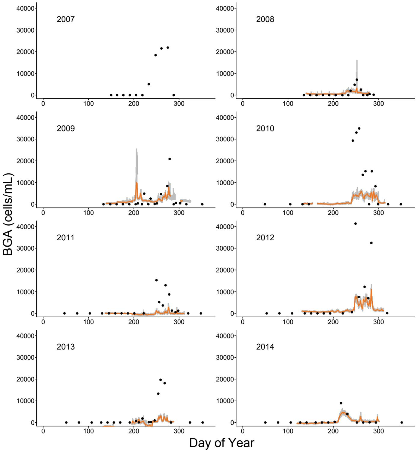
Figure A7. Raw data (light grey lines) and daily means (orange line) of blue-green algae (bga) cell density estimates from the phycocyanin probe located below near Turwar. Black points indicate bga cell density from grab samples taken near the sonde location.
