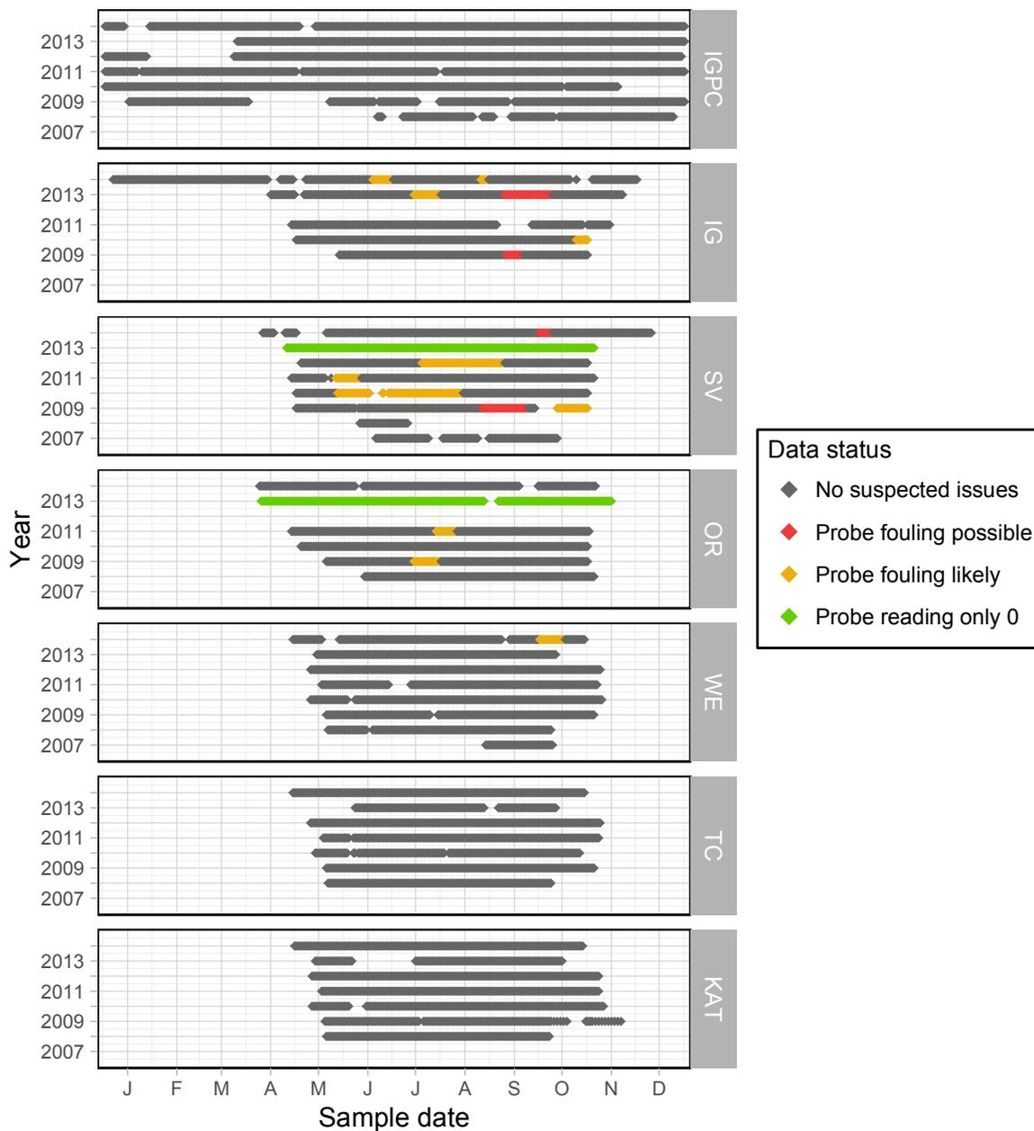
Figure 2. Timing of sonde BGA measurements by year and day at the seven long-term sonde sites on the Klamath River below Iron Gate Dam from 2007 to 2014. Red, yellow, and green points are days with quality assurance concerns. Month abbreviations on the x-axis are at the 15th of each month.
