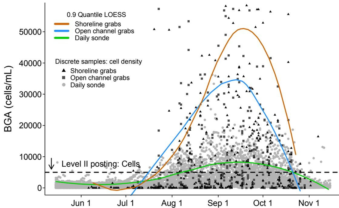
Figure 8. BGA cell density by date from shoreline grabs (SL), open channel grabs (OC), and daily mean sonde BGA (as reported from YSI phycocyanin probes). Lines show the 0.9 quantile LOESS fit for each data type and dashed lines show the Tribal level II public health advisory for cell density.
