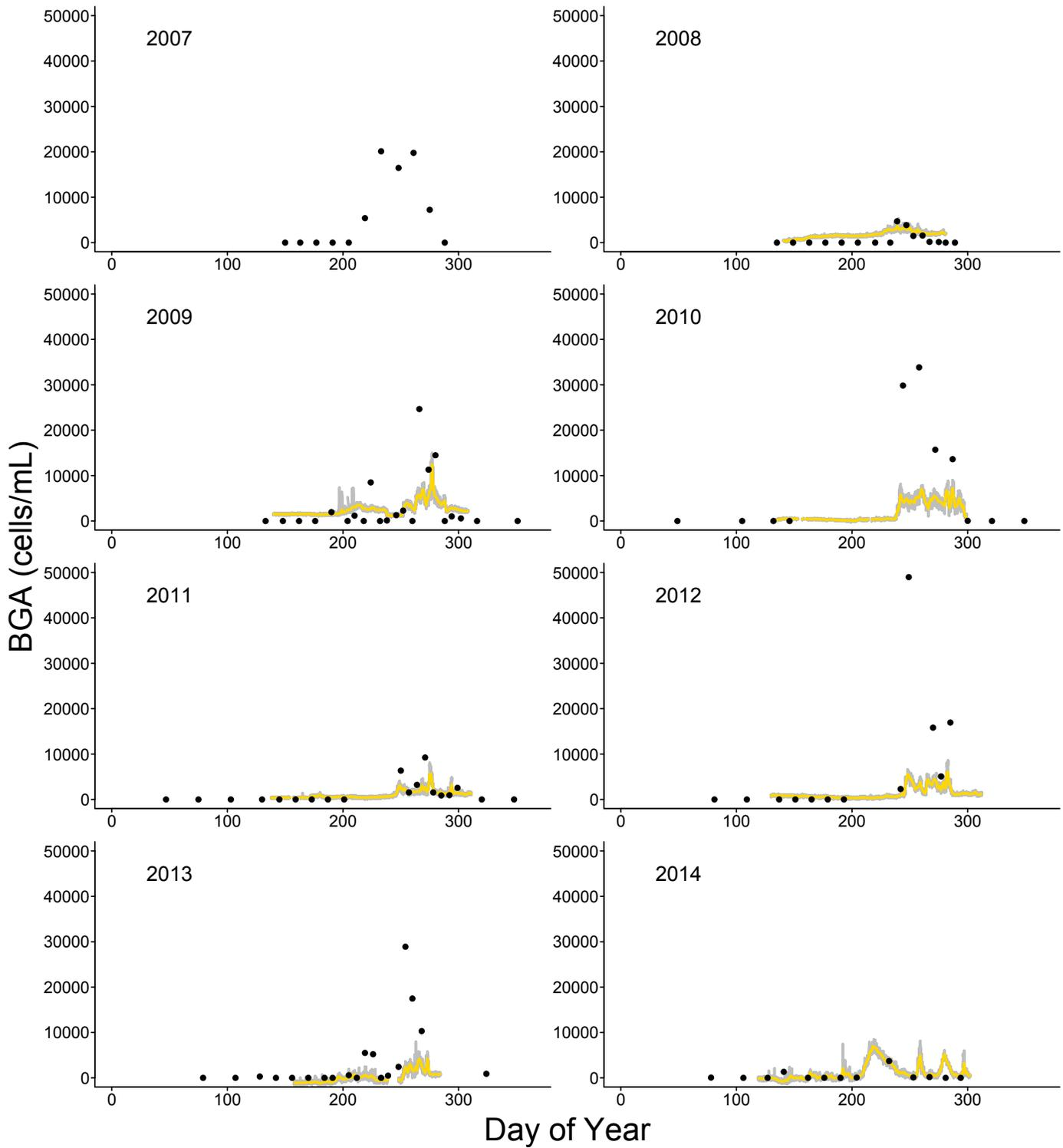
Figure A6. Raw data (light grey lines) and daily means (yellow line) of blue-green algae (bga) cell density estimates from the phycocyanin probe located below Tully Creek. Black points indicate bga cell density from grab samples taken near the sonde location.
