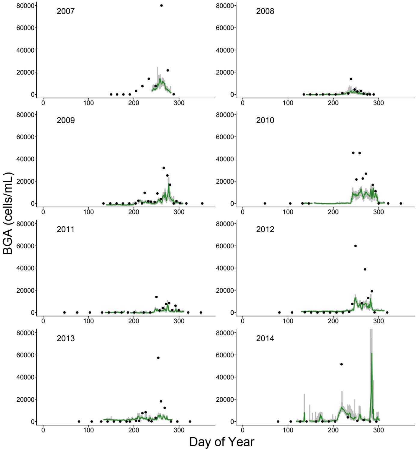
Figure A5. Raw data (light grey lines) and daily means (green line) of blue-green algae (bga) cell density estimates from the phycocyanin probe located near Weitchpec. Black points indicate bga cell density from grab samples taken near the sonde location.
