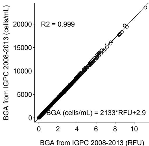
Figure 3. Daily mean sonde BGA (cells/mL) from the Iron Gate sonde operated by Pacifi Corp from 2008 to 2013 as predicted by the daily mean of sonde BGA (RFUs) reported the same day.
