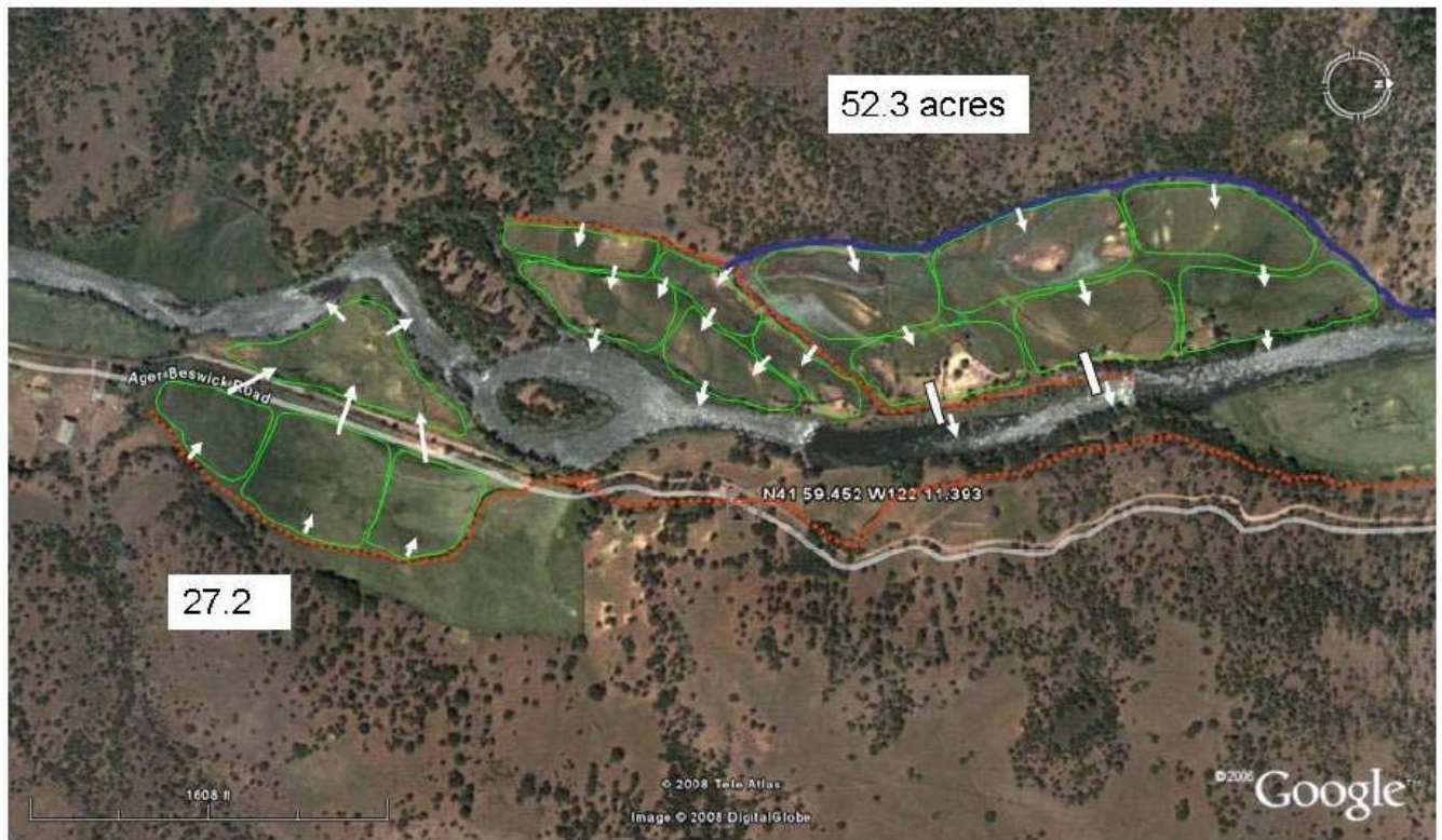
Figure 3. A gently-sloping area on PacifiCorp’s ranch upstream of Copco reservoir that is suitable for placement of constructed wetlands. Figure from Lyon et al. (2009), accompanied by the following caption: “Conceptual layout of surface flow wetlands at Site 013 on the Klamath River upstream of Copco reservoir. As much as possible, this makes use of the pre-existing gravity fed canals (in red) and when necessary, installs new channels (in blue).”
